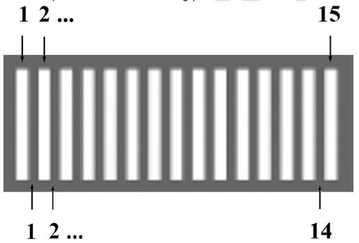
3. Place test chart on flat surface below camera so the test bars are in a vertical orientation (see figure above). The camera back must be parallel to this surface.
