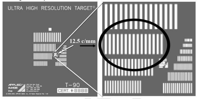
Visually verify (count) the number of dark and light lines and record each (e.g., 15 light and 14 dark – See figure below). It is recommended that a magnifier or loupe be used in the counting process.
