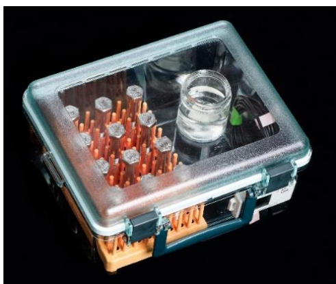
Figure 2. Photographs of the enclosures used to control the environmental conditions for DNA sample exposure. These enclosures are simple and cost-effective to maintain. (A) Image of enclosure used to control temperature and relative humidity. This enclosure is shown with the stainless steel bolts in place. Bolts were spaced evenly on a peg rack. (B) Image of the enclosure used for ultraviolet (UV) light exposure. This enclosure is shown with the cotton fabric squares in place. Fabric squares were pinned to cork baseboard to enable even exposure of all surfaces to UV light. A light fixture containing UV bulbs was rested on support blocks at the top of the UV enclosure. Both enclosures housed glass beakers filled with saturated salt solutions to maintain constant humidity levels, and probes to monitor temperature, humidity, and UV light levels.
