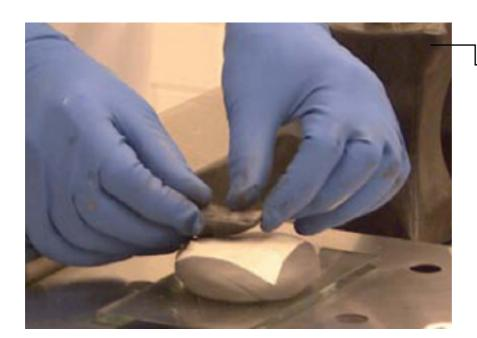
Lifting sheet is placed on top of duct seal. (Photo courtesy of the FBI Latent Print Unit.)
