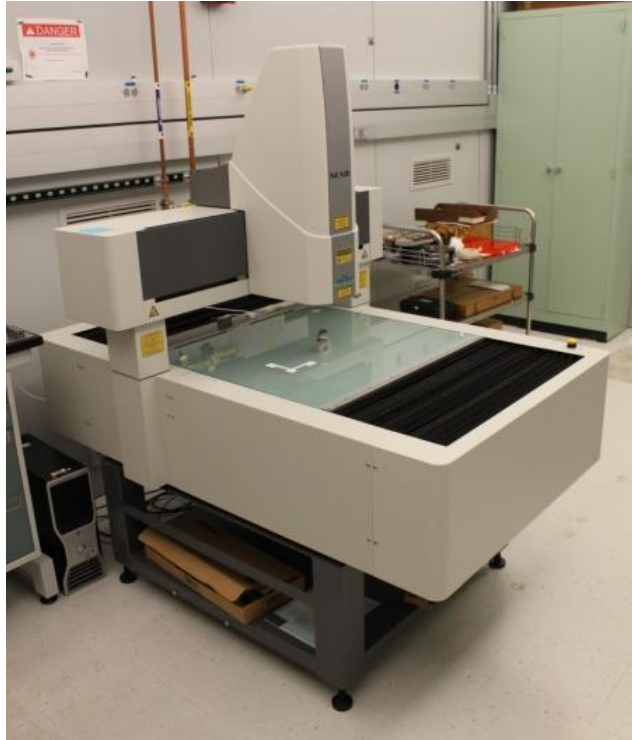
Figure 6: The Nikon VMR-6555 was purchased in 2008 and was used for all subsequent measurements in this study.
