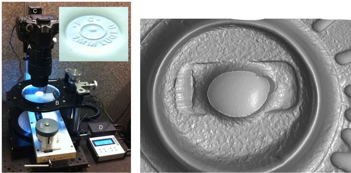
Figure 3: TopMatch-GS 3D Scanner. (Left) The current capture setup contains an 18-megapixel Canon EOS Rebel T3i digital camera with a 65mm macro lens (A), GelSight elastomeric sensor (appears as a white disk through glass) (B), glass light-plate with embedded electronics (B), motorized camera control (C), electronics control box (D), cartridge case holder and mount (E). (Inset) View of case as seen through gel. (Right) Surface rendering of the 3D measured surface of a Glock fired casing. The impressed breech-face impression and striated primer shear marks are clearly present. Note that the firing pin impression was not imaged and may thus look unusual to a firearms examiner. Images were downsampled for presentation. In the original images, a single pixel corresponds to 1.4\mu\text{m} .
