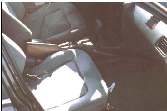
Photographing into a vehicle with existing light — exposures with strong sunlight entering a vehicle compartment usually result in photographs with deep shadows. Detail in the deep shadow areas may not be recorded on the film.
