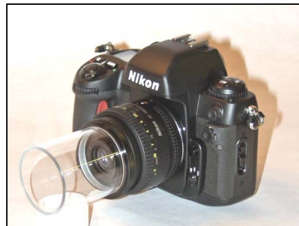
1:1 adapter screws onto the front of the camera's normal lens.
