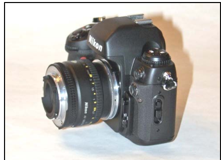
Reverse-mounting the lens creates magnification.
