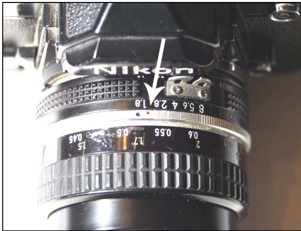
Infrared focusing mark (indicated by arrow) on a standard lens.
