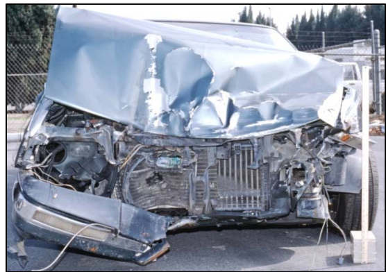
Collision damage photographed with electronic flash — shadows are filled in with lighting to reveal the extent of the damage.
