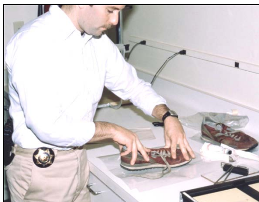
The ink is transferred from the shoe sole to a clear sheet of plastic.
