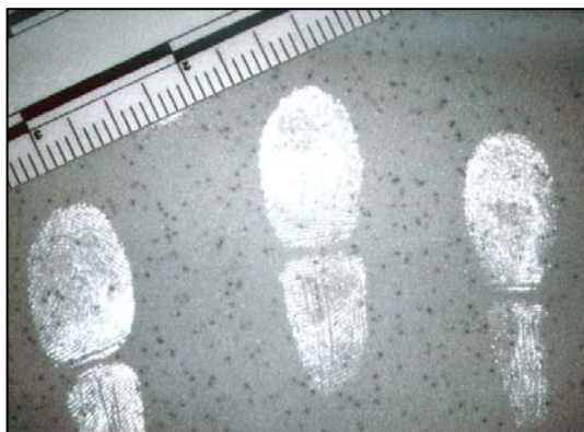
Fingerprints dusted with fluorescent powder and illuminated with a forensic light source. An orange filter was used over the lens.
