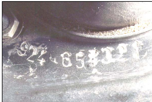
Stamped or engraved serial numbers are photographed using oblique lighting.
