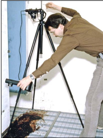
When photographing bloodstain evidence use a scale on the same plane as the bloodstain and photograph with the film plane parallel to the plane of the bloodstain. Use oblique lighting.
