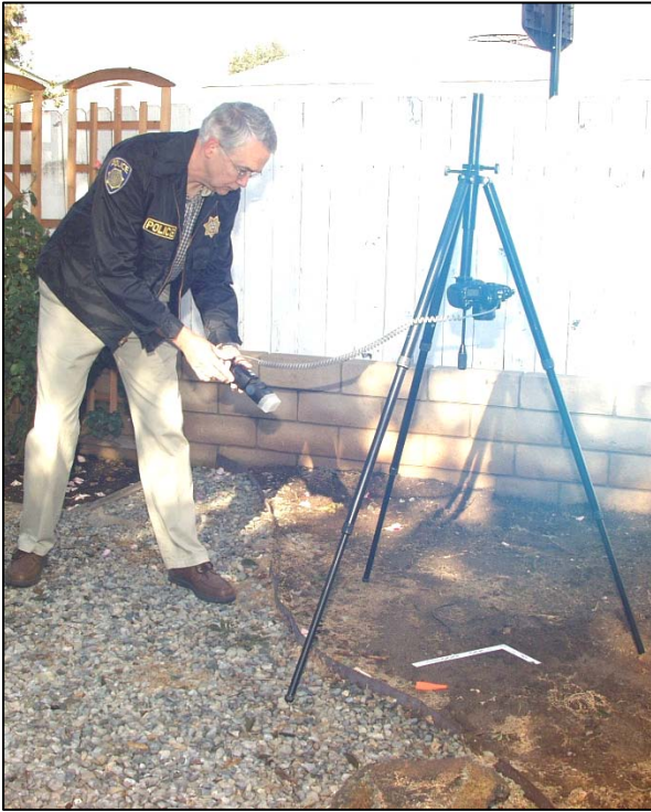
Photographing impressions — use a scale on the same plane as the impression. Keep the film plane parallel to the plane of the impression. Position the electronic flash or light source at angles that highlight the detail in the impression. Preview the photograph by using a strong light source at different angles.
