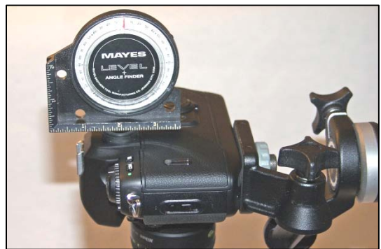
An angle finder can be used to position the camera so the film plane is parallel with the impression. Measure the angle of the impression and then adjust the camera to the same angle.
