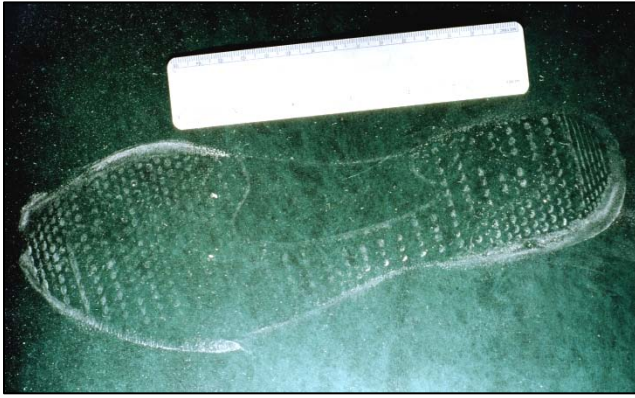
Dusty footwear impression left on a vinyl chair — nearly invisible to the naked eye, this impression was photographed using a low oblique light angle. Photograph by Joe Brown, University of California Davis Police Department.
