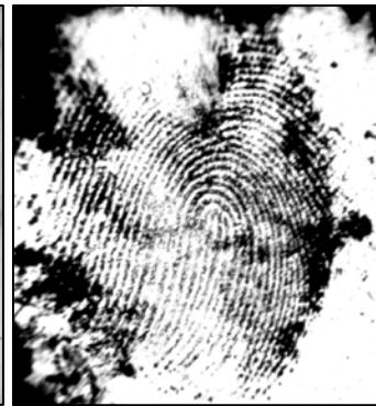
High contrast film was used to photograph the same faint, dusted fingerprint.
