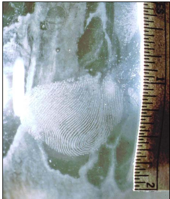
Fingerprint on drinking glass using transmitted lighting — position a diffused light source behind the glass.
