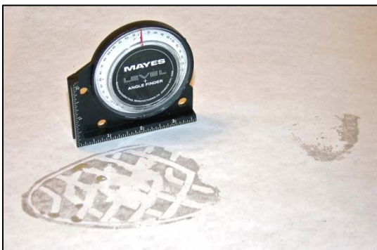
An angle finder can be used to position the camera so the film plane is parallel with the impression. Measure the angle of the impression and then adjust the camera to the same angle.
