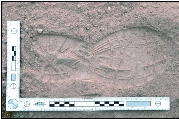
Place the scale approximately one inch away from the impression and on the same plane as the impression.
