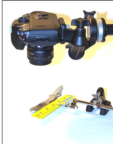
Proper scale position for photographing evidence. The scale is positioned on the same plane as the evidence.
