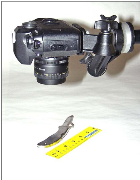
Improper scale position for photographing evidence. The scale not positioned on the same plane as the evidence (a fingerprint on the knife handle).
