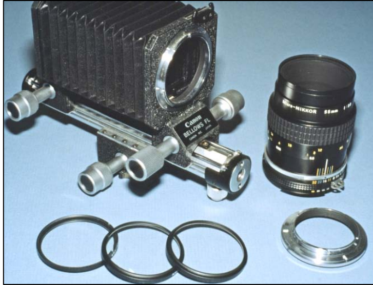
Close-up Equipment — clockwise from top left: bellows, macro lens, reversing ring, close-up filters
