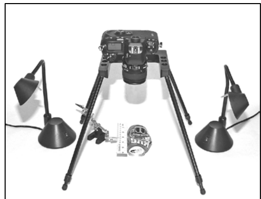
A portable copy stand or a tripod can be set up at the crime scene to photograph evidence.
