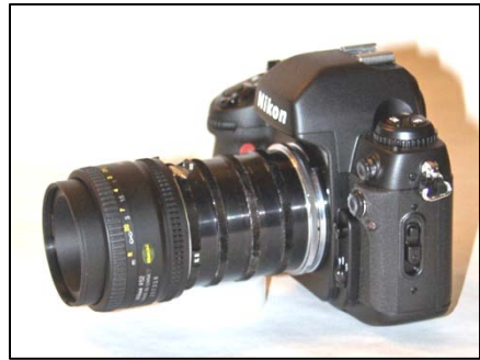
Extension tubes are placed between the camera body and the lens to increase magnification.
