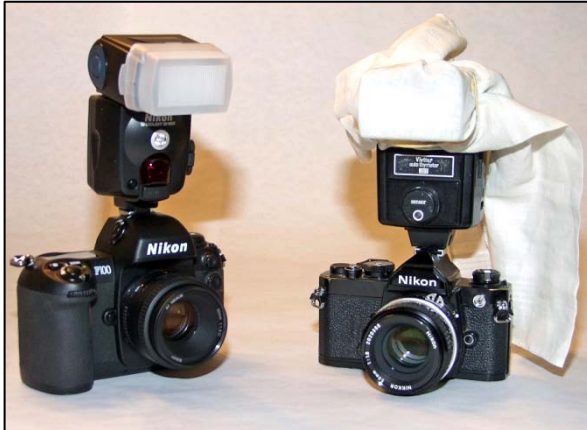
A wide angle diffuser or handkerchief over the flash head will soften the light from an electronic flash.
