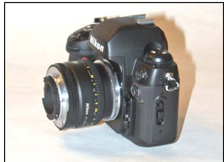
Reverse-mounting the lens creates magnification.
