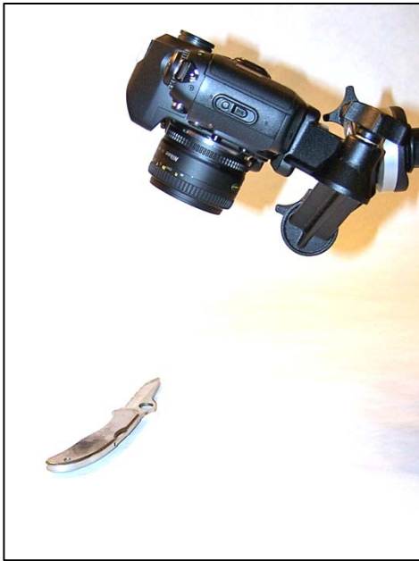
Improper camera position for photographing evidence. The camera is positioned at an oblique angle to the evidence.
