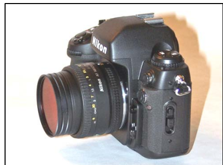
Close-up filters screw on the front of a normal lens to provide increased magnification.
