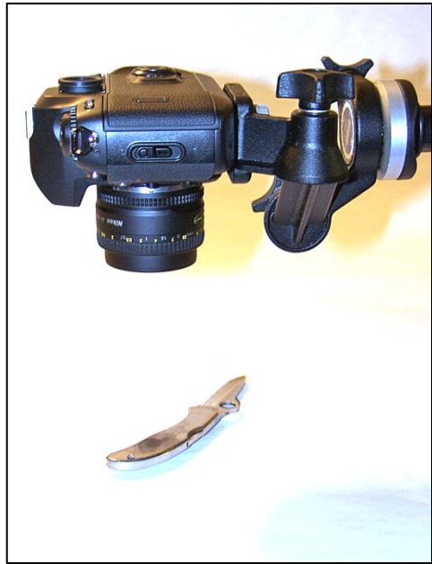
Proper camera position for photographing evidence. The camera's film plane is parallel with the evidence.
