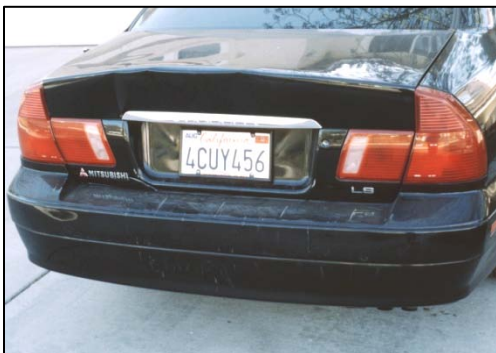
A vehicle struck from the rear received minor damage. An imprint in the dust on the rear bumper shows the other vehicle's license number. The dust imprint was photographed at the scene with diffused side lighting.
