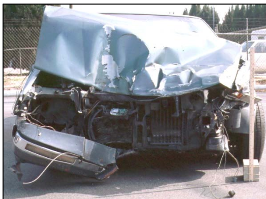
Collision damage photographed with normal lighting — shadows conceal the extent of the damage.
