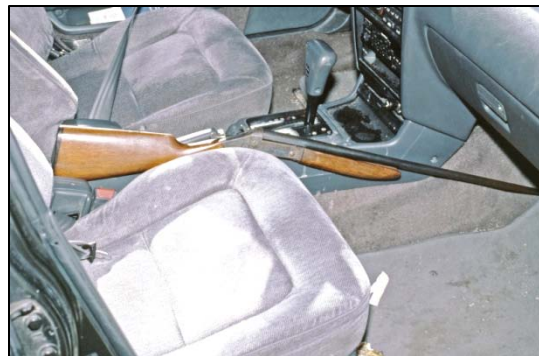
Photographing into a vehicle using electronic flash — detail in the deep shadow areas is recorded. Electronic flash is also useful for photographing into vehicle trunks and engine compartments.
