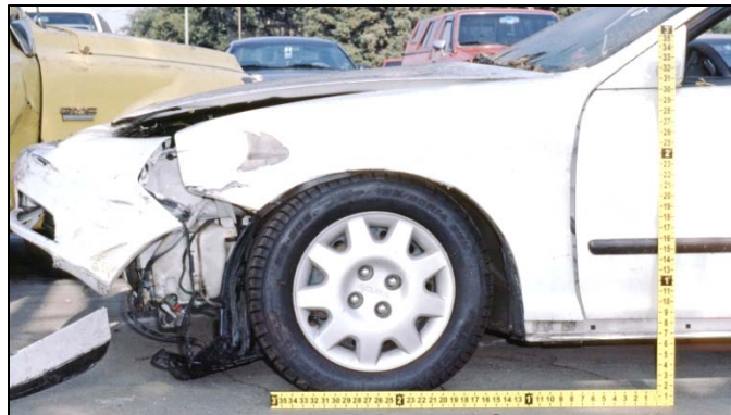
When photographing collision damage, use an electronic flash to fill in shadows and scales with large, easy to read numbers.
